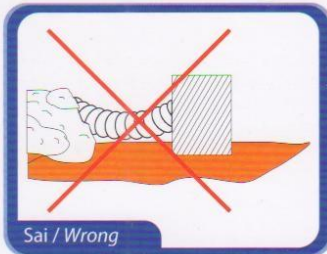
Khi lắp, tránh làm võng đường ống. Don't cause BFP conduits to sag, deform during trench filling.
